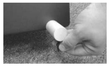
stop. Carefully tilt the tower speaker to one side and screw the metal spikes into the bottom of the front and rear aluminum stabilizer bars (at least 3/8") to the desired height. Hand tighten the nut to lock it in position. When both sides are installed, check to ensure that the speaker does not rock. If necessary, tilt the speaker, loosen the nut and adjust the height until the speaker rests firmly on all four spikes. You can use a small wrench to further tighten the nuts.
